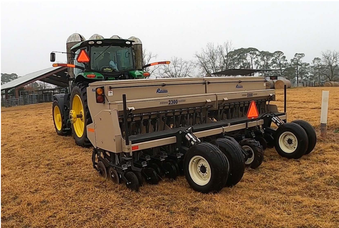
No-till drill used to plant seeds of different sizes.
